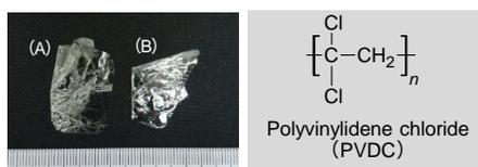
**Method** ionRocket combined with QTOF-MS equipped with DART ion was used as analytical system for this application (Fig. 2). A small piece of sample (ca. 0.5 mm<sup>2</sup>) was put into the ionRocket sample POT. A temperature gradient of 100 °C/min. from room temperature to 600 °C was applied (total run time: 7 min.).
