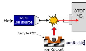
Fig. 2 : ionRocket DART-MS system
