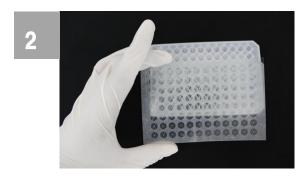
Paste the RAPID SlitSeal on the 96-well plate and make sure holes of RAPID SlitSeal are correctly positioned on each well spot.
